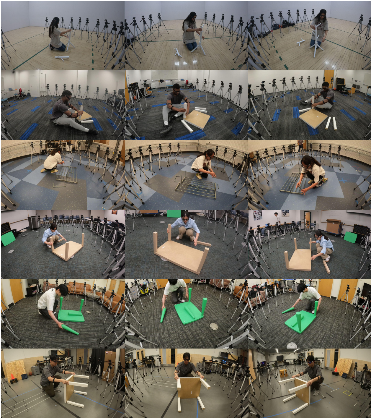
Figure 1. Multi-View Capture System. From a single view, finger keypoints are extremely challenging during object manipulation due to severe occlusion. Our multi-view system makes joints blocked from one viewpoint can be seen from another, and therefore is able to provide accurate joint annotations.
