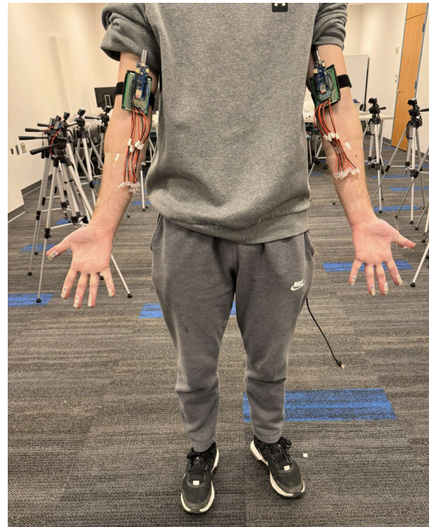
Figure 4. The Arduinos are secured on the individual's upper arms using loop straps, and sponges are affixed beneath each Arduino to serve as a medium. The sensor will be covered by the sleeves and remain mostly invisible during the capture.
